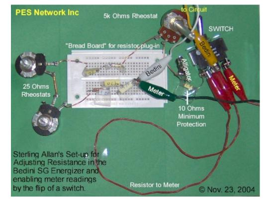
The 25 Ohm resistors give a fine-tuning capability. The bread board enables hard resistor plug-in to the appropriate range desired. The 5k Ohm potentiometer enables a wide berth of tuning.
