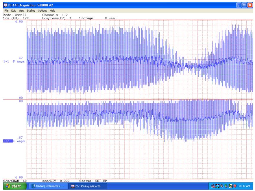
SSG w/Board 1; Wheel 2 – Gap 0.365" w/o Resistor 246 RPM – depicts transition zones denoted by Amp spikes at 164, 227,257 rpm
