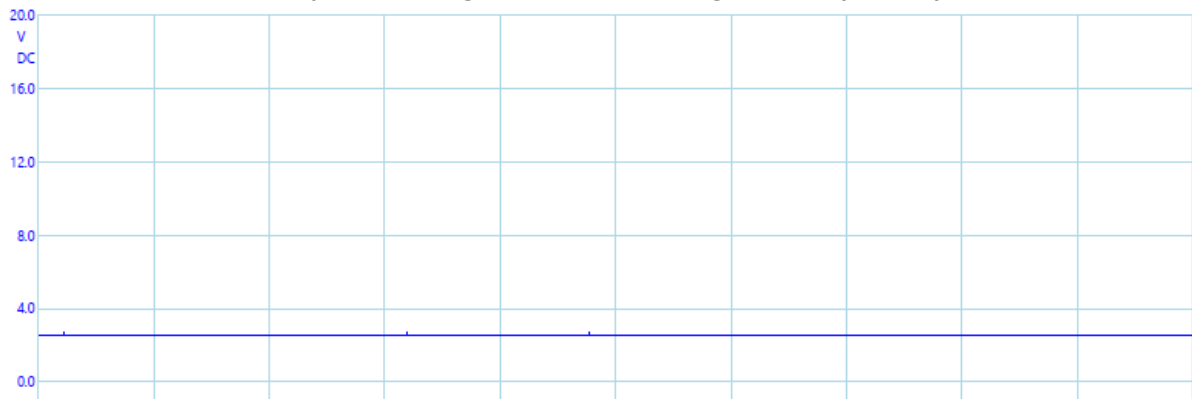
Capacitor voltage BEFORE connecting secondary battery
