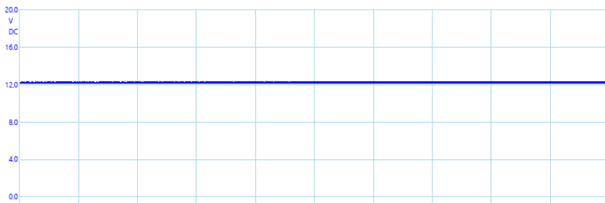
Capacitor voltage AFTER connecting secondary battery
