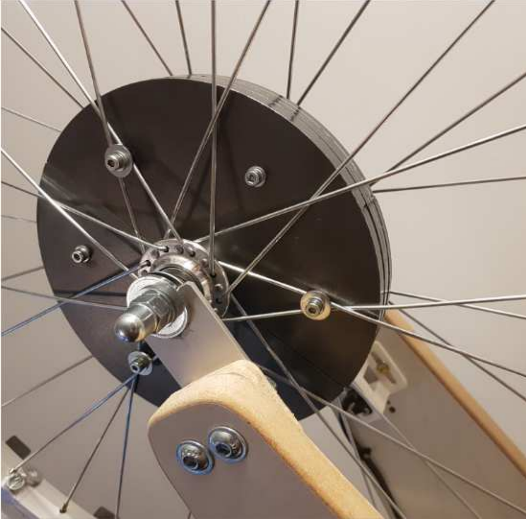
5kg "Flywheel" added to rotor
