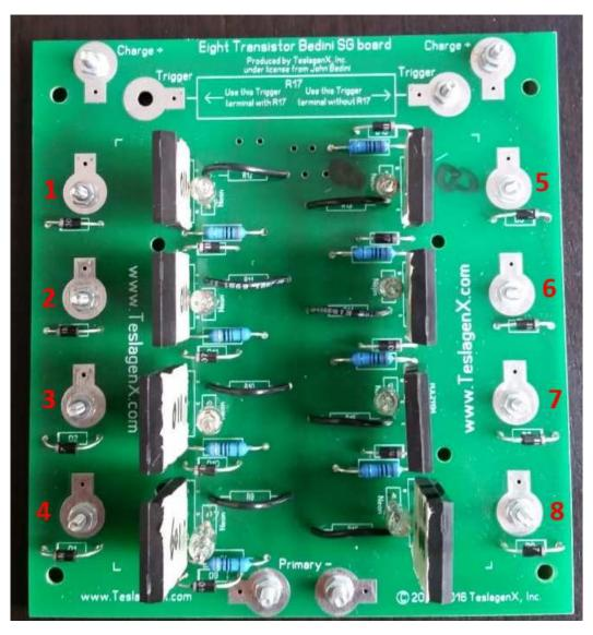
Radiant mode, 12mm gap, LA1@input, A@output, 7 power coils. Input +/-1amp Prope 1: ground to negative of input battery, positive to collector transitor 1 Prope 2: ground not connected, positive to collector transitors 2,3,4,5,6,7
