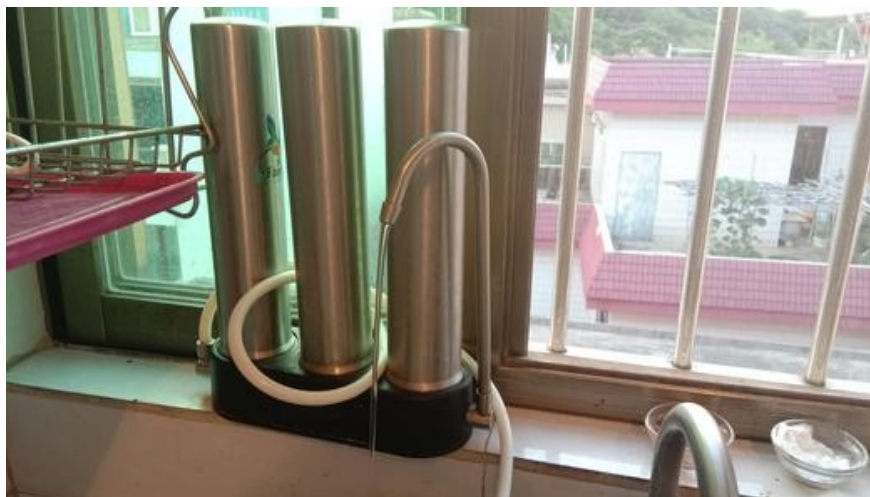
Three stages (ceramic, activated carbon, ceramic+silver) tap water filter.
